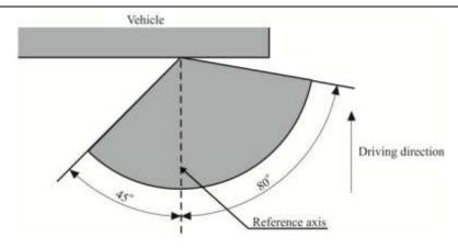
However, in the case where a device is intended to be installed with its H plane at a mounting height less than 750 mm above the ground, the inward angle of 45° may be reduced to 20° under the H plane.
