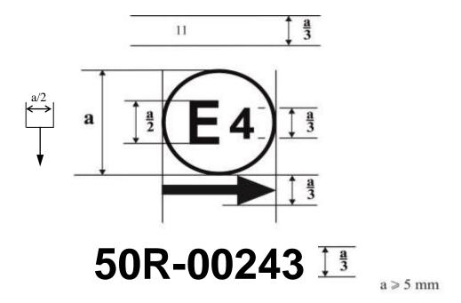
A device bearing the approval mark shown above is a direction indicator of the category 11 approved in the Netherlands (E 4) under the number 00243. The first two digits of the approval number indicate that the approval was granted in accordance with the requirements of Regulation No. 50 in its original form.
