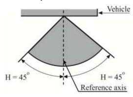
However, in the case of a pair of lamps, the inboard geometric visibility requirement is deemed to be satisfied if the lamps conform to the photometric values prescribed in the field of light distribution for the approval of the device."
